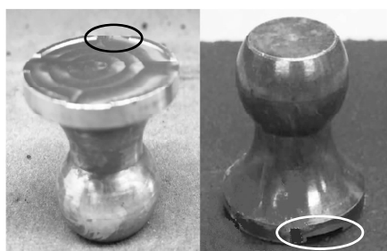
(a) Pull-off stubs with overflow weirs in BBS test
