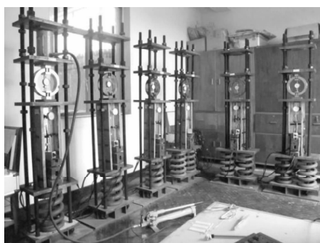
图4 长期荷载施加现场 Fig. 4 Applying long-term loads on site
