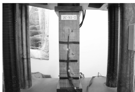
图5 长期荷载卸载后的二次加载试验 Fig. 5 Secondary static loading test after long-term loading
