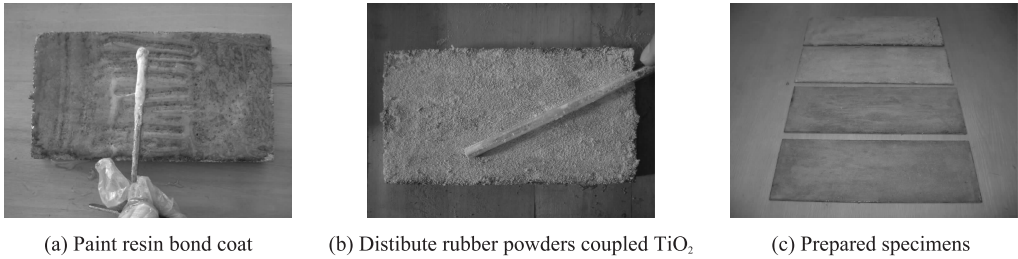
图 1 试件制备过程 Fig. 1 Specimen prepared process
