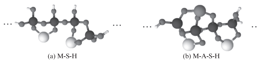
图6 M-S-H和M-A-S-H的单层结构示意图 Fig. 6 Single layer structure diagram of M-S-H and M-A-S-H
