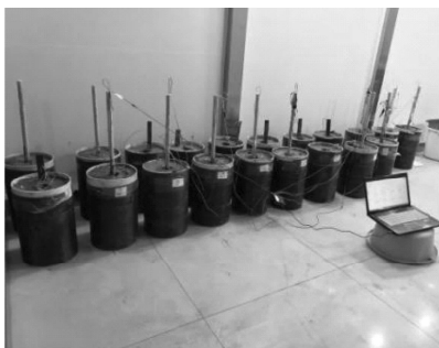
图 2 含膨胀锚固体的土样试件 Fig. 2 Soil sample with expansion anchor solid
