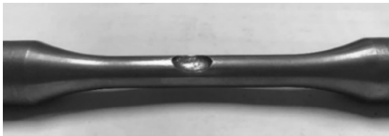
(a) Corrosion morphology of steel bar
