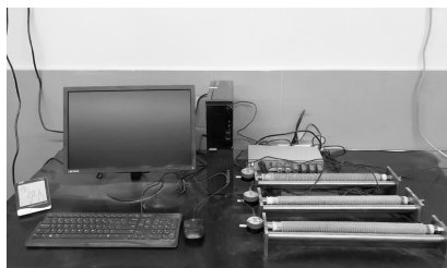
图2 水泥净浆自收缩和干燥收缩测试仪器 Fig. 2 Equipment for measuring autogenous and drying shrinkage of cement paste
