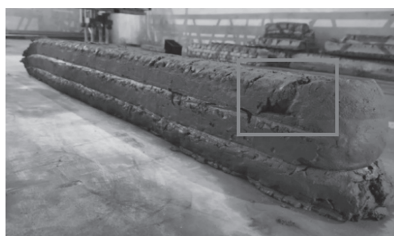
(b) 3D printable SAC filament
