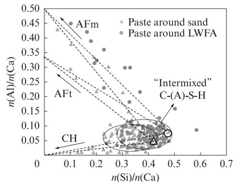
图3 轻集料UHPC的 $n(\text{Al})/n(\text{Ca})$ 与 $n(\text{Si})/n(\text{Ca})$
